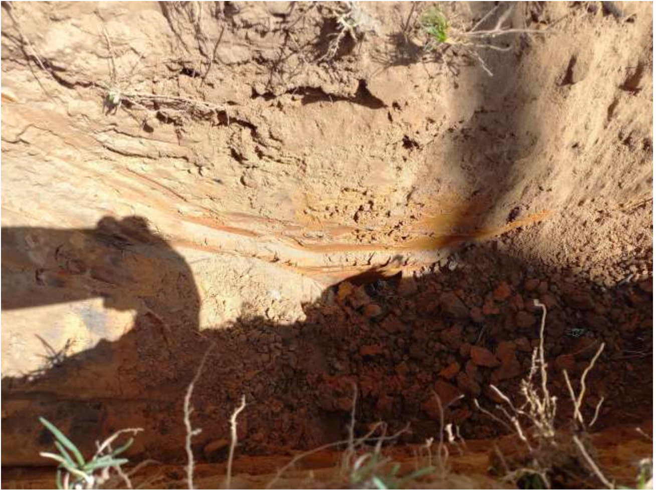
Photograph 3: Test Pit TP103 showing representative soil profile present across the site.
