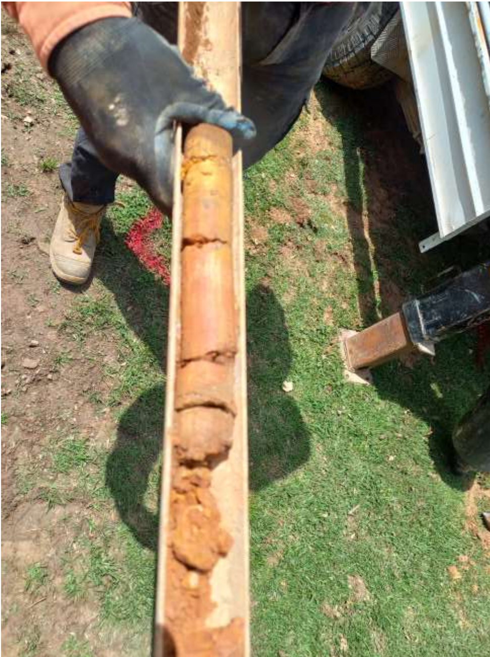
Photograph 4: Borehole BH103 showing representative natural material across the site – silty clay overlaying weathered sandstone
